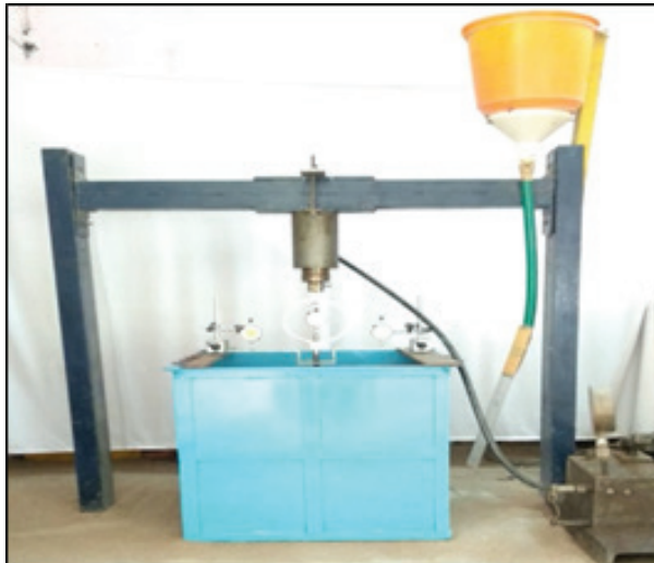
Fig. 2 Experimental Test Setup for Pile Load Test
