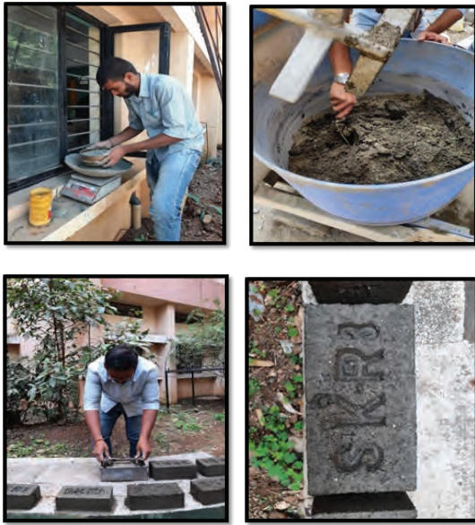
Figure 4. Preparation of mortar bricks
