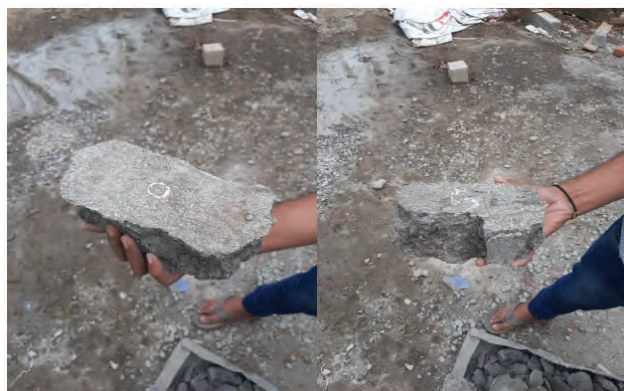
Fig. 5. Bricks after compression test
