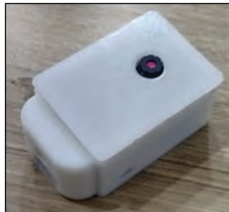
Fig. 9 ESP32 Cam with 3D Enclosure
