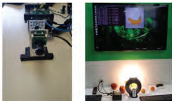
Fig. 2. Ongoing connection setup with AR 1335 13 MP associated with NVIDIA Jetson Xavier
