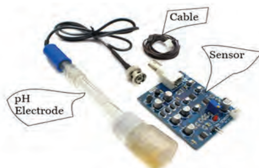
Fig. 3. Kit for measuring pH using a traditional glass electrode sensor
