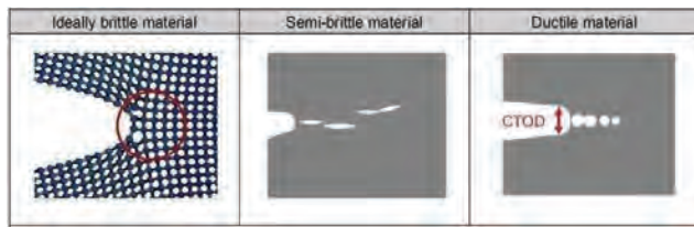
Fig. 1 Crack propagation in three different type of materials (Pippan et al, 2018)
