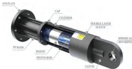
Fig. 2. Fluid viscous damper
