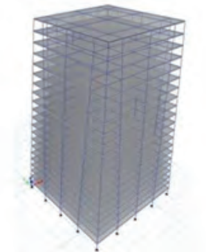
Fig 4. Multi-storeyed building with oblique columns ( 82^\circ )
