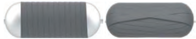
Fig. 3: (a) Hoop and (b) Helical winding[37]
