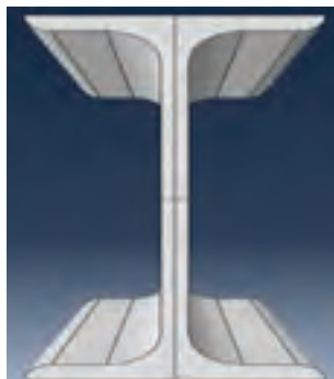
Fig. 5 Cross sectional view of standard I-section
