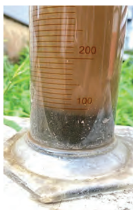
Fig. 3: a) Floc formation b) Sludge settlement
