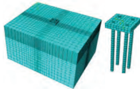
Fig. 6. 3D view of pile group modelled with pile diameter=0.7m, pile length = 9m
