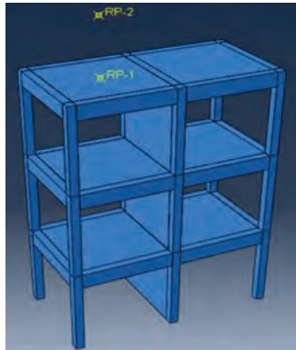
Fig. 7 RC frame with shear wall and frame with shear wall
