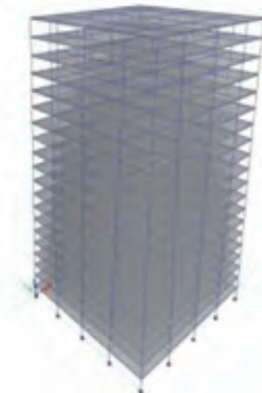
Fig. 5. Multi-storeyed building with oblique columns ( 85^\circ )
