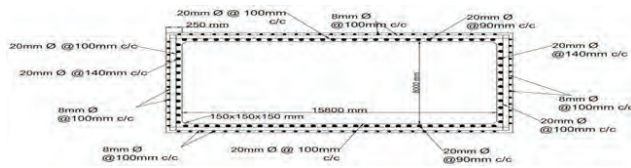
Fig. 1: Reinforcement detailing of water tank (top view)
