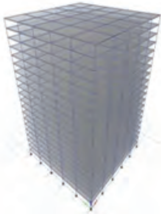
Fig. 7 Multi-storeyed building with conventional columns (90°)
