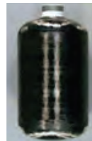
Fig. 2: Composite Overwrapped Pressure Vessel[31]
