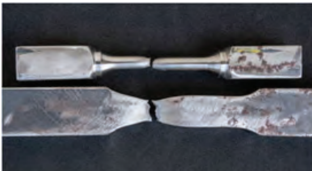
Fig. 2 Ductile Damaged Specimens [15]
