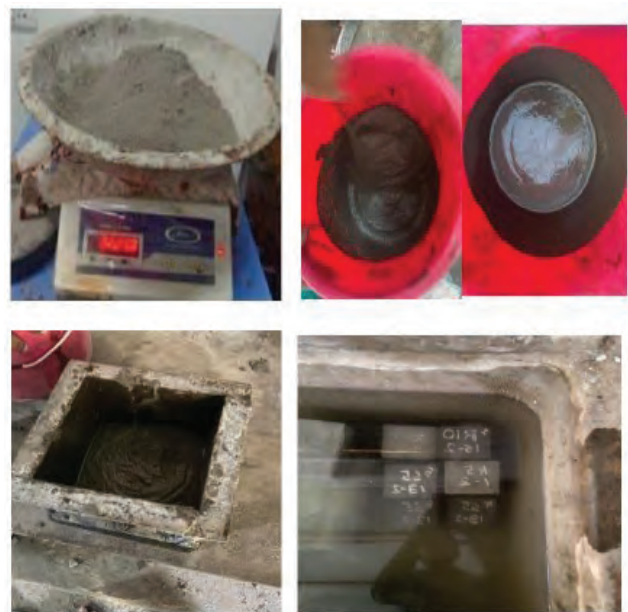
Fig. 1 Batching, Mixing, Placing of FC, Curing of FC
