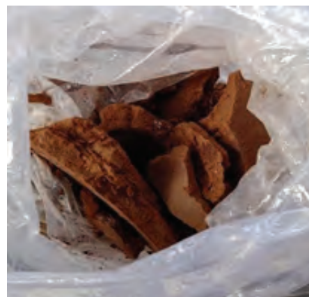
Fig. 2 Aluminium Based Sludge
