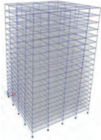
Fig. 6 Multi-storeyed building with oblique columns (88°)
