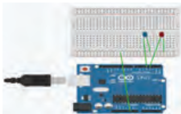
Fig. 5 Transmitter module with circuit
