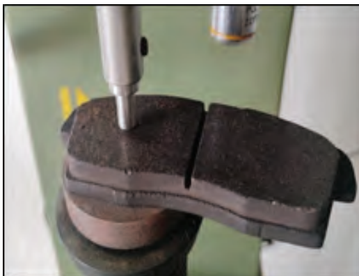
Fig 6: Hardness Test of Existing Brake Pad
