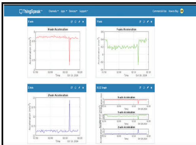
Fig. 3 Visualization of vibration data (X, Y, Z axes) on ThingSpeak
