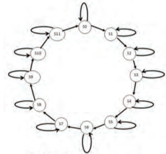
Fig. 3: State diagram of traffic light controller
