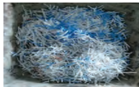
Fig. 2: Fibers extracted from empty cement bags
