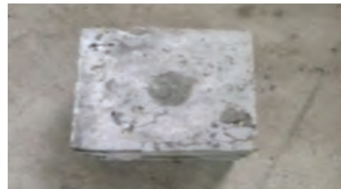
Fig. 5: Concrete Specimen after compressive strength test
