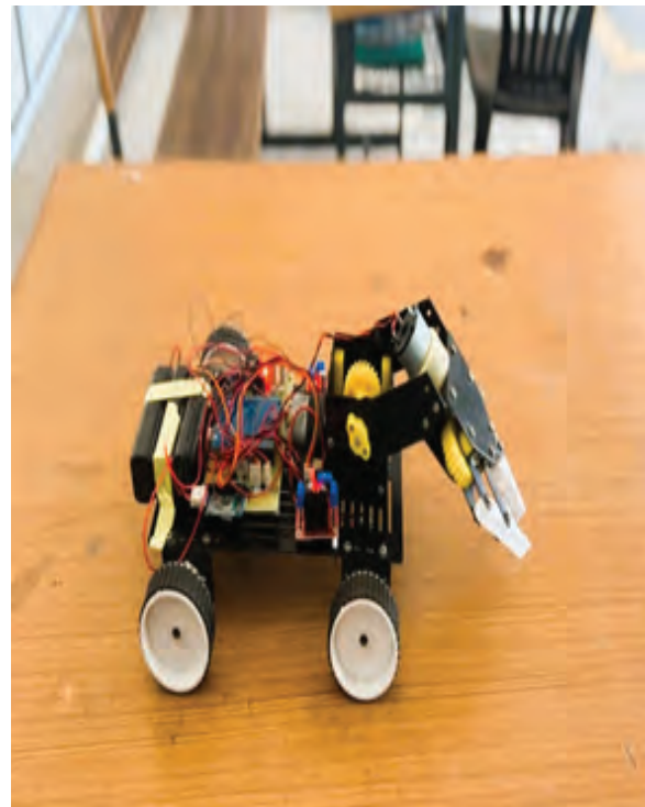
Fig. 4: Actual Setup of the Pick and place ROBOT
