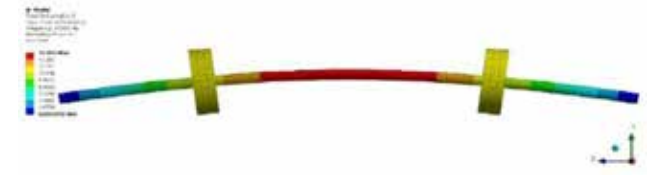
Figure 7. Modal analysis of Steel shaft two disk system
