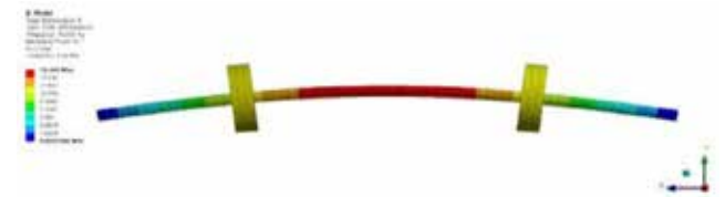
Figure 5. Modal analysis of Aluminum shaft Two disk system
