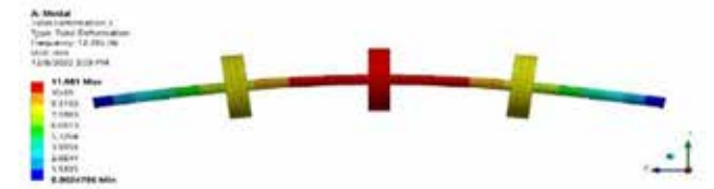
Figure 6. Modal analysis of Aluminum shaft Three disk system
