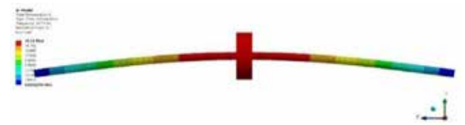
Figure 4. Modal analysis of Aluminum shaft Single disk system
