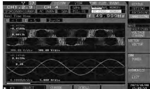
Figure 10: Output parameters of VVVF fed induction motor drives dynamic performance at 75% load
