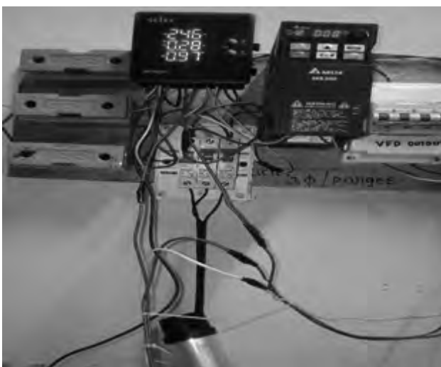
Fig. 5 Phase to neutral voltage, Phase current and PF with reactive load situation
