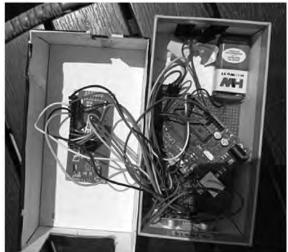
Figure 6. Connections and preliminary hardware prototype of digital measuring tape
