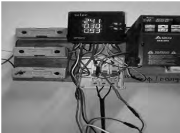
Fig. 4 Phase to neutral voltage, Phase current and PF without reactive load situation
