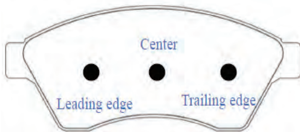
Fig. 7 Wear measurement locations on the brake pad surface
