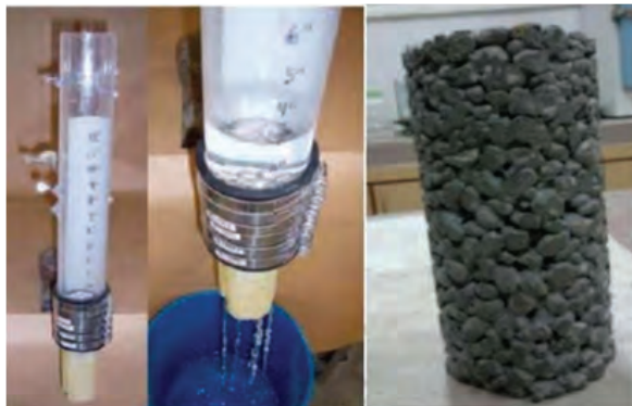
Fig. 9. Porosity Test Setup
