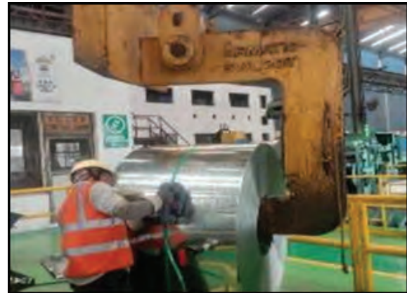
Fig. 2 (a) BOF Operation was monitored through a transparent glass window panel (b) PET strapping of coil ( Source: Tataseel, Kalinganagar)
