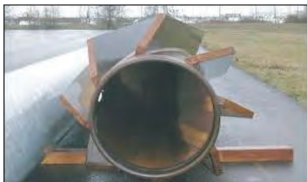
When observed from head to tip, the top of one fin contacts the bottom of the fin next to it, as shown in Figure 2, which illustrates the fins' 360-degree coverage. Fins are easy to install after being bought or built on-site. When connected to the pile cap and serving as an anchor, the uplift capability is much enhanced compared to a pipe alone. By expanding the gross bearing area at the pile's base, the fins also increase end-bearing capacity. Because of this, the compression and tensile capacities of Spin Fin piles are usually attained at less depths than those of straight pipe piles of comparable size. This massive project is being worked on at the moment.
