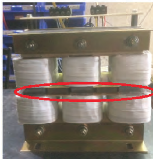
Fig. 2 Special design of core and windings in transformer
