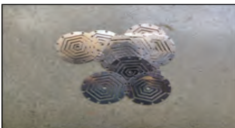
Fig. 11 Manufactured Flexure bearing discs
