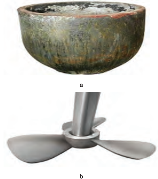
Fig 10. (a) Ceramic Crucible; (b) Stirrer with Three Blade Impeller
