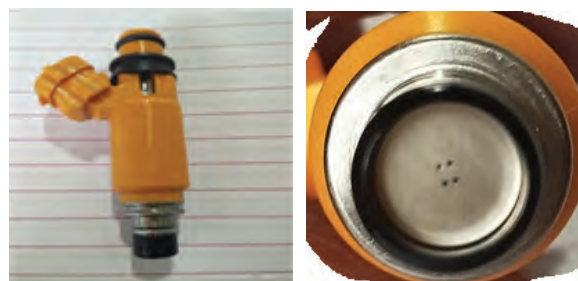
Fig. 4: Saturated Port/manifold (LRF) Liquid Injector
