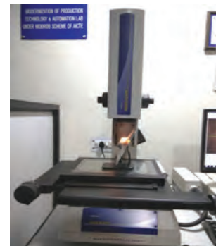
Fig. 3 Strain assessments with 3D microscope
