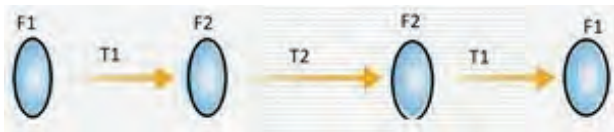
Fig. 6-A: Proposed Cloaking System With A Series of Four Converging and Diverging Lenses
