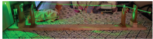
Fig. 6-C: Proposed Cloaking System With A Series of Four Converging Lenses In Night Mode
