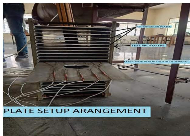
Fig. 2 Experimental Plate Test Set Up
