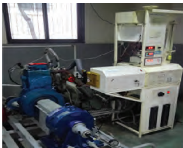
Fig. 1: Engine setup to run the RCCI combustion process
