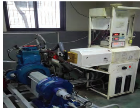
Fig. 1: Engine setup to run the RCCI combustion process
