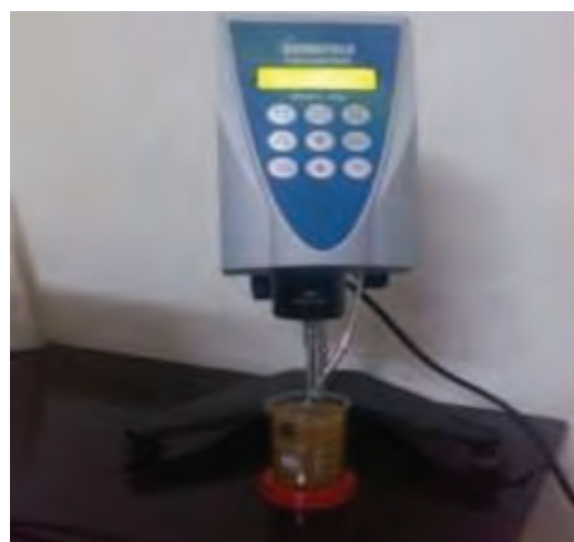
Fig. 2: Viscosity determination by Brook field viscometer
