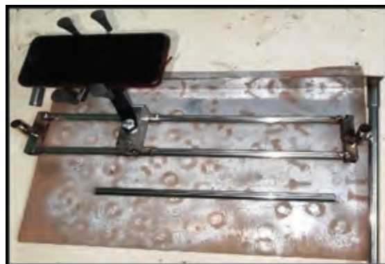
Fig. 4 : Adjustable height and position for Camera in Upward – Downward and left - Right Direction
