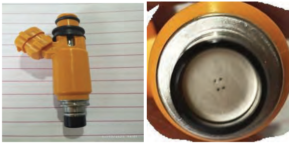
Fig. 4 Saturated Port/manifold (LRF) Liquid Injector
