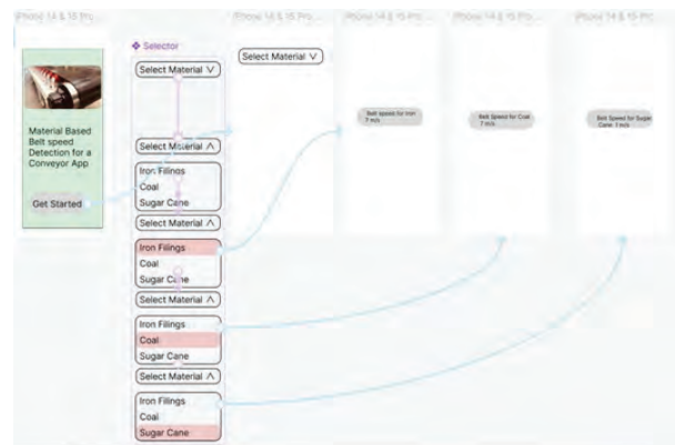
Fig. 9: Prototype of Design of UI for Material based Automatic belt speed selection from the results of AIML based Multiple Linear Regression Model using Figma
