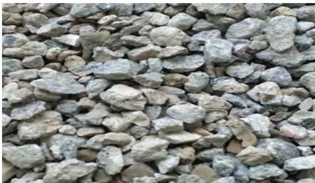
Fig. 2 Recycled Concrete Aggregates
