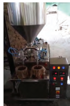
Fig. 4 Jaggery filling LCA workstation
