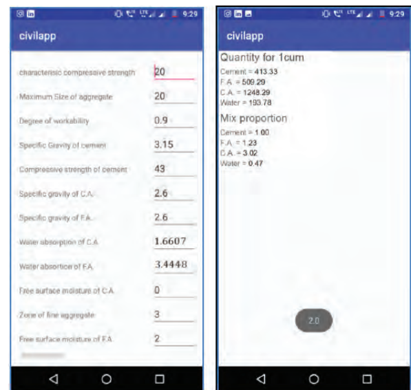
Fig. 2: Mix Design Result from Android Application
