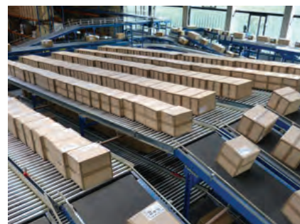
Fig. 1: A typical industrial roller conveyor
