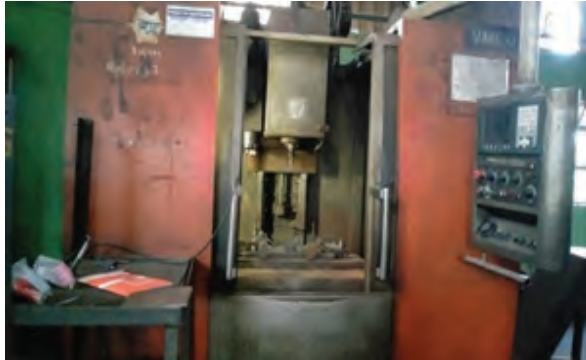
Fig 4: Vertical Machining Center (VMC) machine
