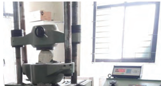
Fig. 5: Split tensile strength of cylindrical specimen
