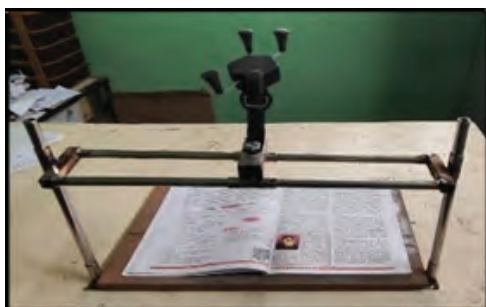
Fig. 3: Foldable, Easy to Carry Hardware Assembly Design
