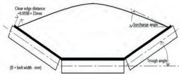
Fig. 4: A three-roll trough idler belt Conveyor
