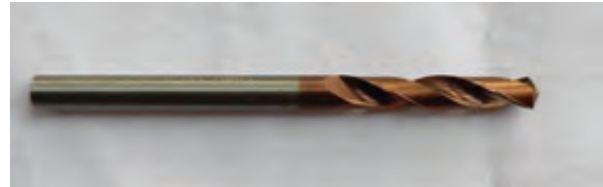
Fig 2: Tool Coated with AlTiSiN
