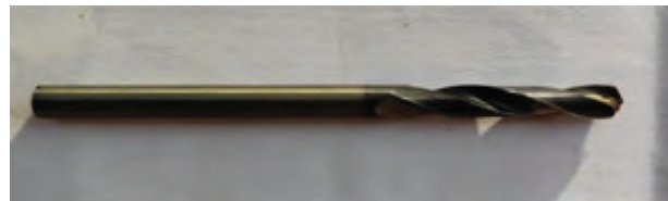
Fig 3: Tool coated with AlTiN
