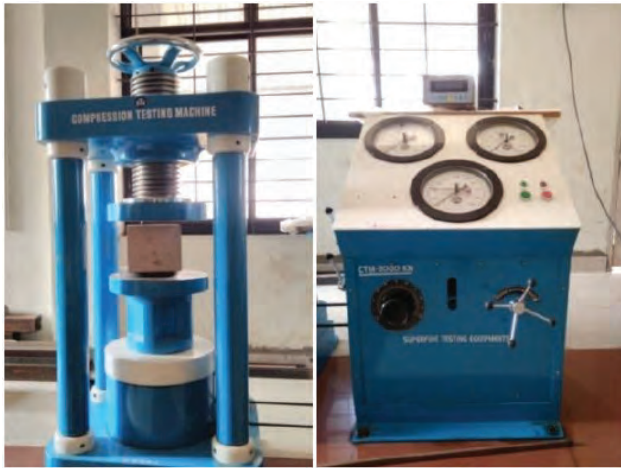
Fig. 3: Compression test of cube specimen
