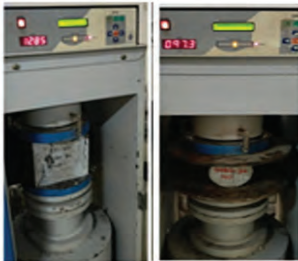
Fig. 4: Cylinder and cube sample testing on a compression testing apparatus
