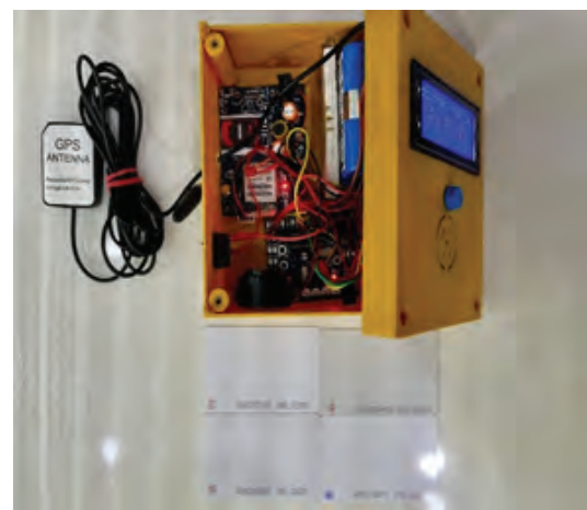
Fig. 3 Encloser Box with System Hardware Assembly and Battery Power Source
