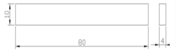
Fig. 8: ASTM D 790 standard flexural specimen
