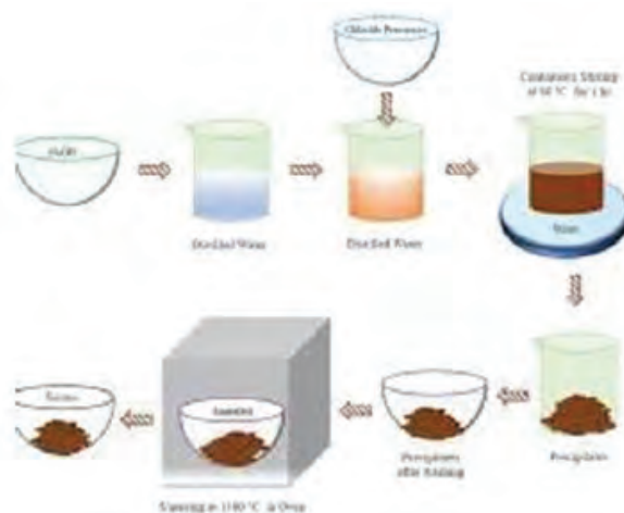
Fig. 3: Synthesis Flowchart in Co-precipitation Method
