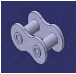
Fig. 4.2: Joint plate and bushing assembly
