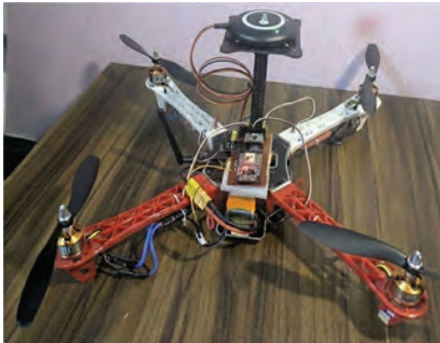
Fig. 7: Assembled quadcopter prototype with custom flight controller
