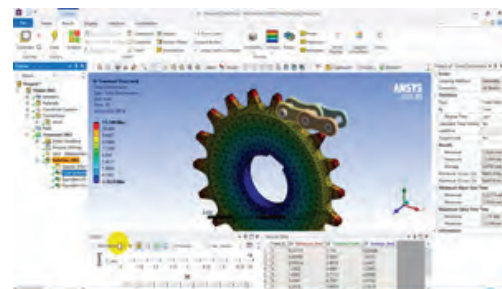
Fig. 4.4: Meshed component of chain sprocket
