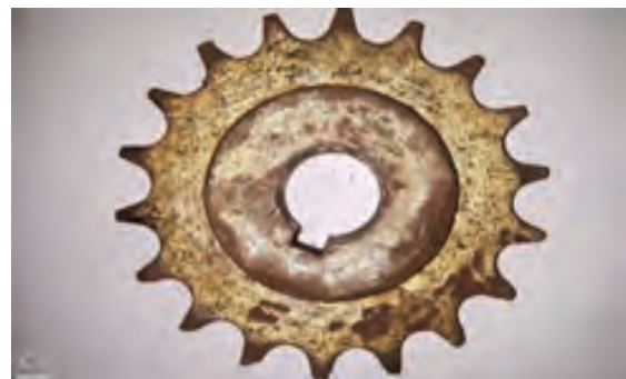
Fig. : Drive side damaged sprocket
