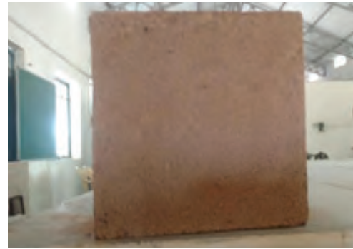
Fig. 10: Foundry sand brick before testing
