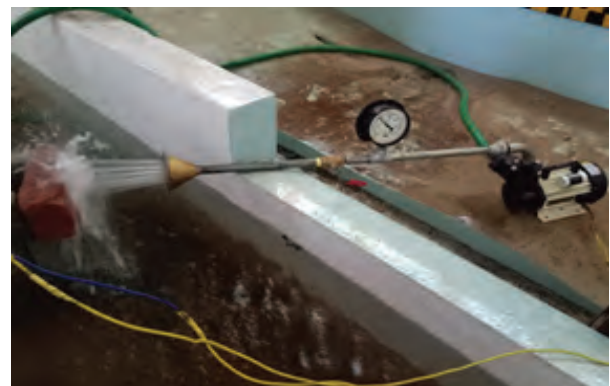
Fig. 7: Accelerated erosion testing apparatus
