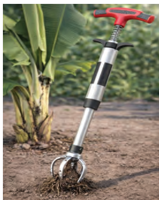
Fig. 7: Real-time field view of the banana shoot sucker extraction device in operation.
