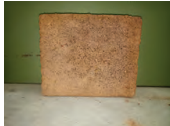
Fig. 11: Foundry sand brick after testing
