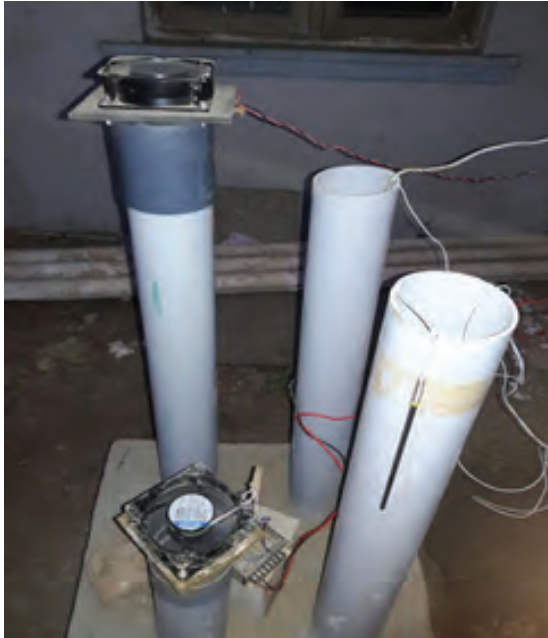
Fig. 11: Experimental setup of vertical BTHE
