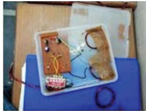
Fig. 6: Prototype design of wireless transmission
