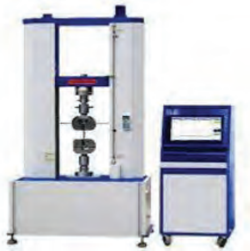
Fig. 4: Tensile Testing Machine Setup
