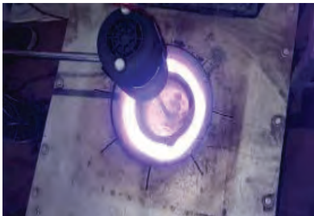
Fig. 2: Stir Casting Setup
