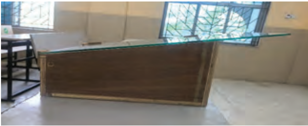
Fig.9: Solar still made of wooden box with glass
