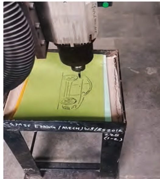
Fig. 5: Toolpath direct deployment to ABB robot
