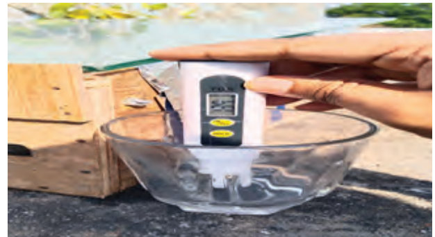
Fig.1 1: TDS testing of saline & desalinated water
