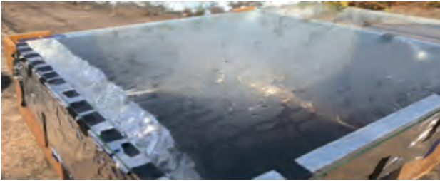
Fig.9: Solar still made of wooden box with glass
