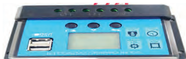
Fig.6: Charge Controller of Battery
