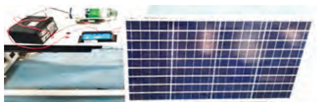
Fig.5: Solar Panel, battery, charge controller &amp; pump
