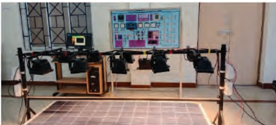
Fig. 6. 260Watts solar PV power Measurement Experimental Setup
