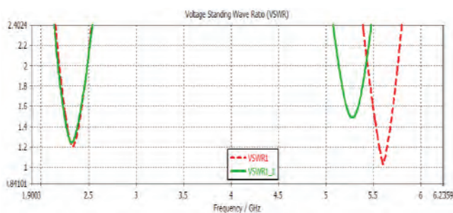
Fig.6. VSWR plot. (Red curve: Conventional design, Green curve: TFSPMA)
