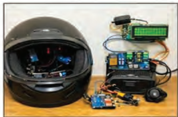
Fig. 6. Experimental setup of the complete system showing the helmet transmitter unit and vehicle receiver module
